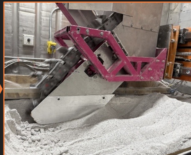
Trencher in test 5 making 1-wall cuts
